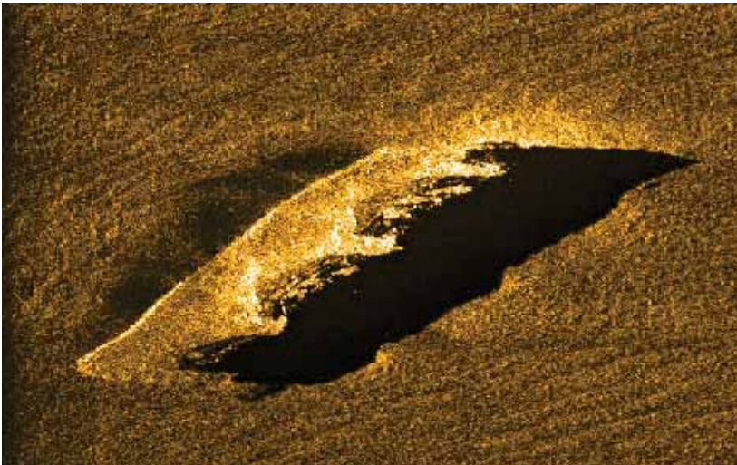
Side scan imagery of redbird subway car
