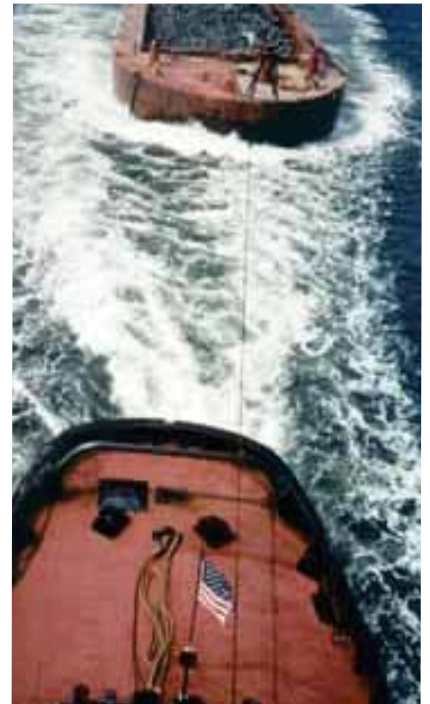
Tug and hopper scow in transit to a reef site for a dredge rock deployment.
