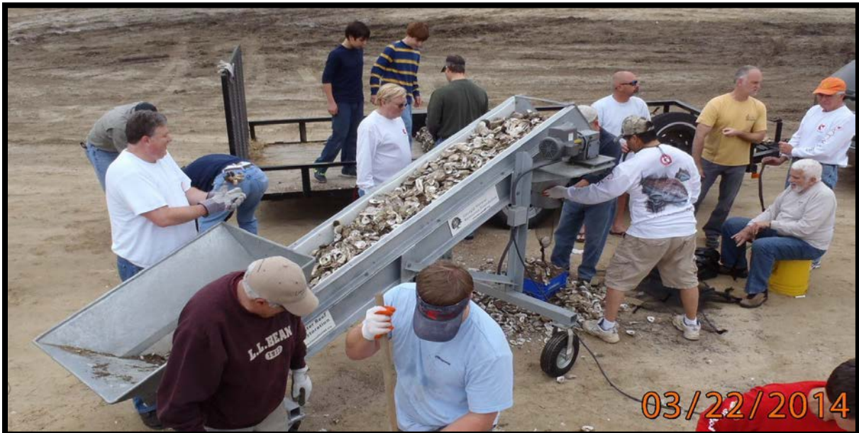
GADNR's oyster shell bagging machine was used in partnership with the Coastal Conservation Association of Georgia to create over 900 bags with 14 volunteers in three hours. The bagging machine consists of a lower hopper filled with shells that travel up a conveyor belt and out of an upper hopper into pre-tied plastic mesh bags. Bags are then passed off for additional tying and are loaded onto a trailer. Photo Credit: January Murray, GADNR.
