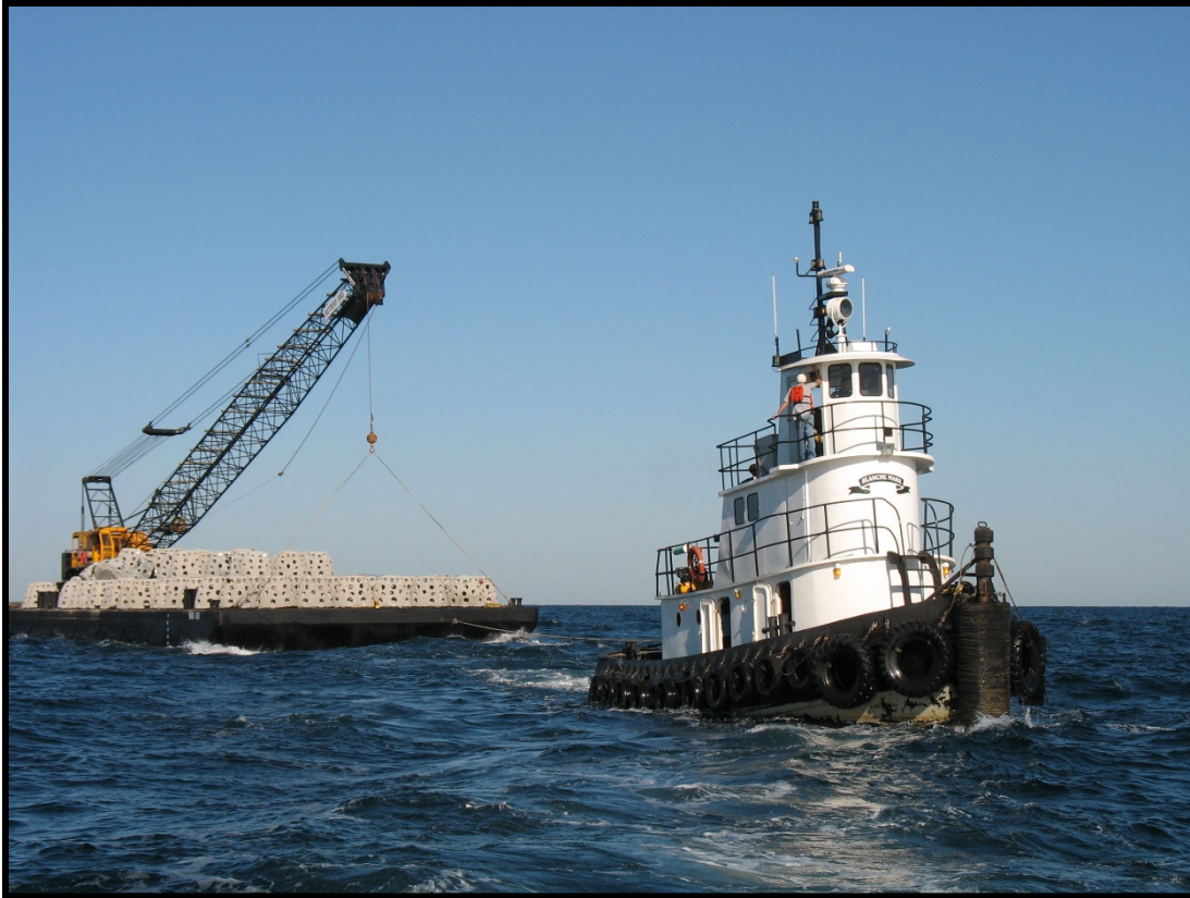
A barge of designed reef modules being transported offshore of Mississippi for deployment. Photo Credit: GSMFC
