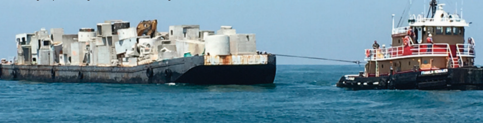
Tugboat positions barge with a load of concrete being added to a reef site.
